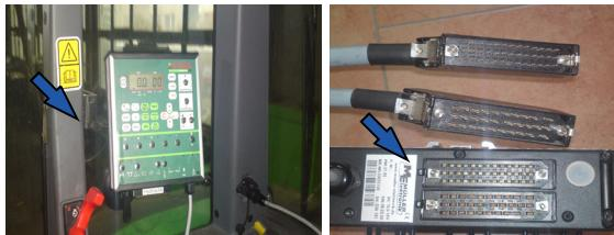
Connection and location of the control panels in the tractor's cabin.
