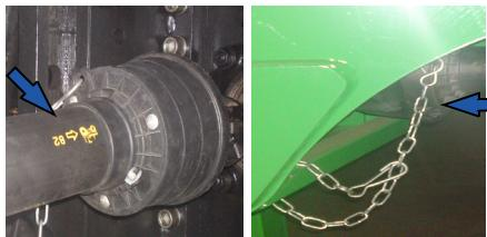
Mount the jointed-telescopic shaft on the end of the sprayer and the tractor.
