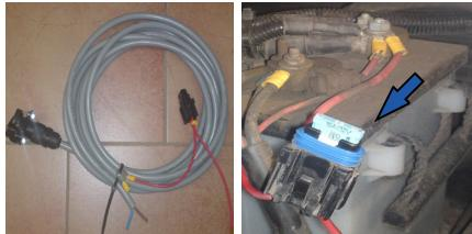
Connect the electrical wiring supplying the control panel to the battery.
