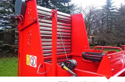
BOLKO is equipped with a potato hopper with the maximum load capacity of 1250 kg. The hopper is unfolded and folded mechanically with a special crank.
