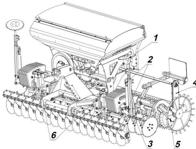
Fig. 19 Lubrication diagram
