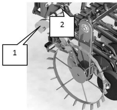
Fig. 1 Retracting the drive wheel
