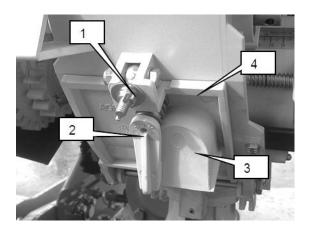
Fig. 14 1 - cover screw; 2- lever of partial pouring off; 3-chute; 4-flap
