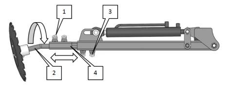
Fig. 17 Adjustment of the track marker
