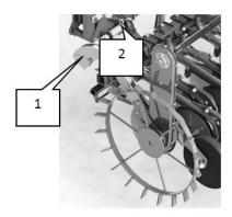
Fig. 1 Retracting the drive wheel 1-drive wheel, 2-securing cotter pins
